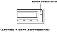
This unit may be controlled from the vehicle's audio controls. An optional Alpine Remote Control Interface Box must be used. For details, contact your Alpine dealer.
